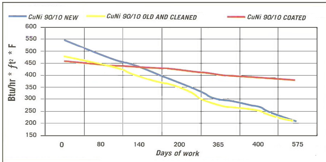
The graph shows the performances over time of coated tubes
